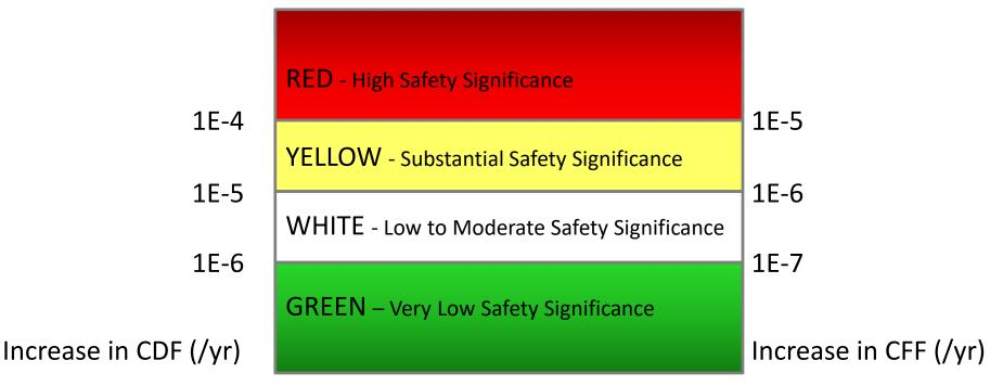
CDF: Core Damage Frequency CFF: Containment Failure Frequency
