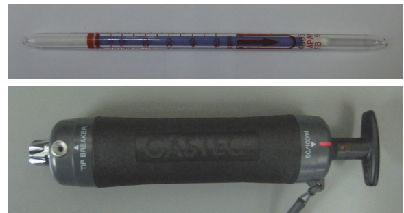
Fig. 2 O 3 detection tube and gas sampler.
