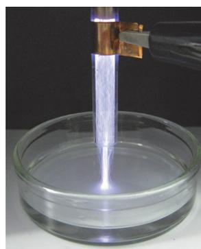
Fig. 2 Plasma jet irradiated onto distilled water.
