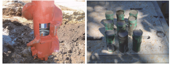
Fig. 2 Sampler and specimen of fresh soil-cement.
