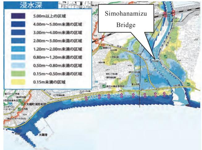
Fig. 8 Inundation prediction result in the Hanamizu River estuary to the assumption tsunami by Kanagawa Prefecture. (The hazard map of Oiso city)
