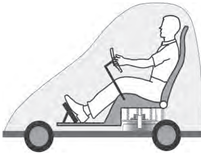
Fig. 1 Intelligent seat completely independent of car body
