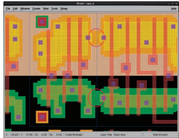
Fig.17 The layout after complement by the our program, complemented area is in the circle red line.
