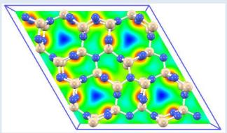
Ab initio calculation result of the atomic arrangement and charge distribution of a silicon nitride crystal with one silicon vacancy. In our laboratory, the electrical and physical properties of novel charge trap materials are also characterized using the new methods which we have developed.
