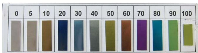
Colored Nb films by anode oxidation method at 0-100V in ammonium borate solution
